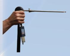
The Sample Conditioning Unit is mounted directly at the sampling probe exit, where excess moisture rapidly condenses and separates from the gas sample. This minimizes contact of the gases with moisture, which could potentially affect NO<sub>x</sub> and SO<sub>2</sub> measurements.
